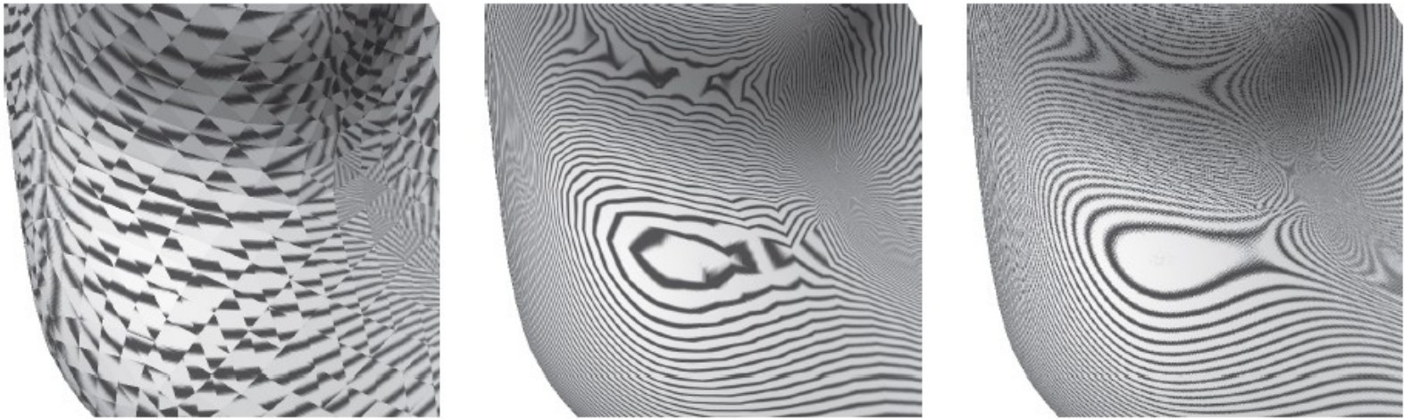
Figure 6.3: Reflection lines on C^0 , C^1 and C^2 surfaces. One clearly sees that the differentiability of the reflection lines is one order lower, i.e., C^{-1} , C^0 and C^1 respectively.
